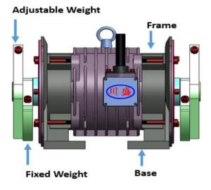
Adjustable weights are attached at both sides and the ends of the shaft. The fixed weight and one adjustable weight are varied. To adjust the vibrating force of CHUAN SHENG Vibrators is simple and easy
